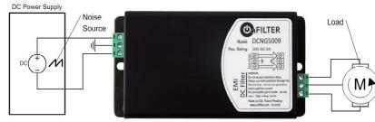
Figure 1. Filter Connection With Noisy Power Source
