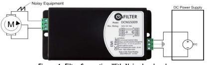
Figure 4. Filter Connection With Noisy Load and One Line Running Through Ground
