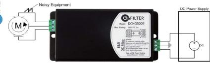
Figure 3. Filter Connection With Noisy Load
